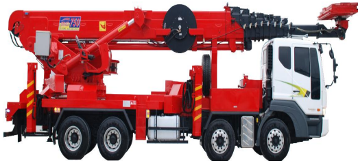
Fig. 1 The aerial work platform of the Electric Work
