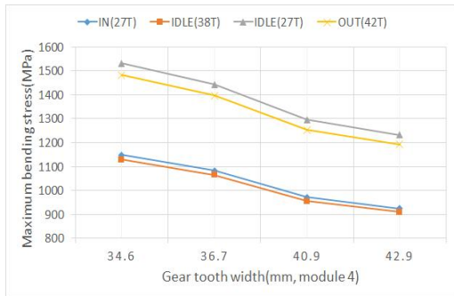
Fig. 4 Stress results according to gear width
