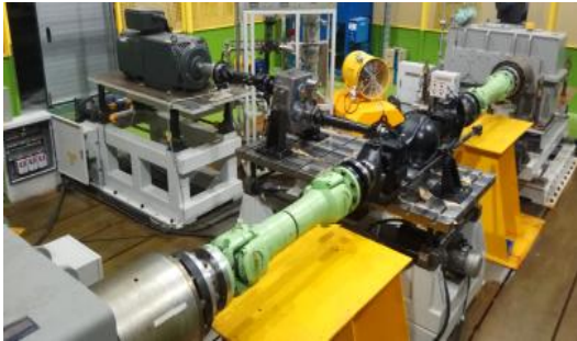
Fig. 9 Durability test set up of the transfer case
