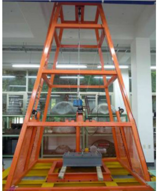
Fig. 2 Free drop collision testing machine
