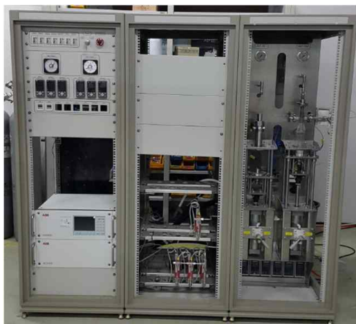
Fig. 3. Urea solution to \text{NH}_3 gasification for catalyst evaluation micro-reactor system.
