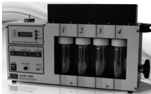
Fig. 5. Marc 7000 Tritium sampler for collecting HTO and HT. The bubblers (No. 1 and 2) cooled to 5\text{-}15\text{ }^{\circ}\text{C} are used to collect HTO. A tubular oven equipped with Pd alumina catalyst pellet heated to 200\text{-}500\text{ }^{\circ}\text{C} to convert HT (as well as hydrocarbon) to HTO, which is collected in bubblers 3 and 4.
