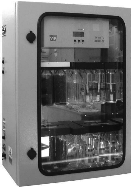
Fig. 6. A tritium and ^{14}\text{C} sampler (V3H14C, VF a.s., Czech Republic) for collecting tritium and ^{14}\text{C} in two fractions. The system includes two parallel lines, the first line equipped with heated platinum catalyst, and the second line without. Each line consists 3 bottles filled with silica gel absorber to trap tritiated water and 3 bottles filled with NaOH solution to trap ^{14}\text{CO}_2 . Therefore, the first line is used to collect all species tritium and ^{14}\text{C} , while the second line is used to collect tritiated water and ^{14}\text{CO}_2 .
