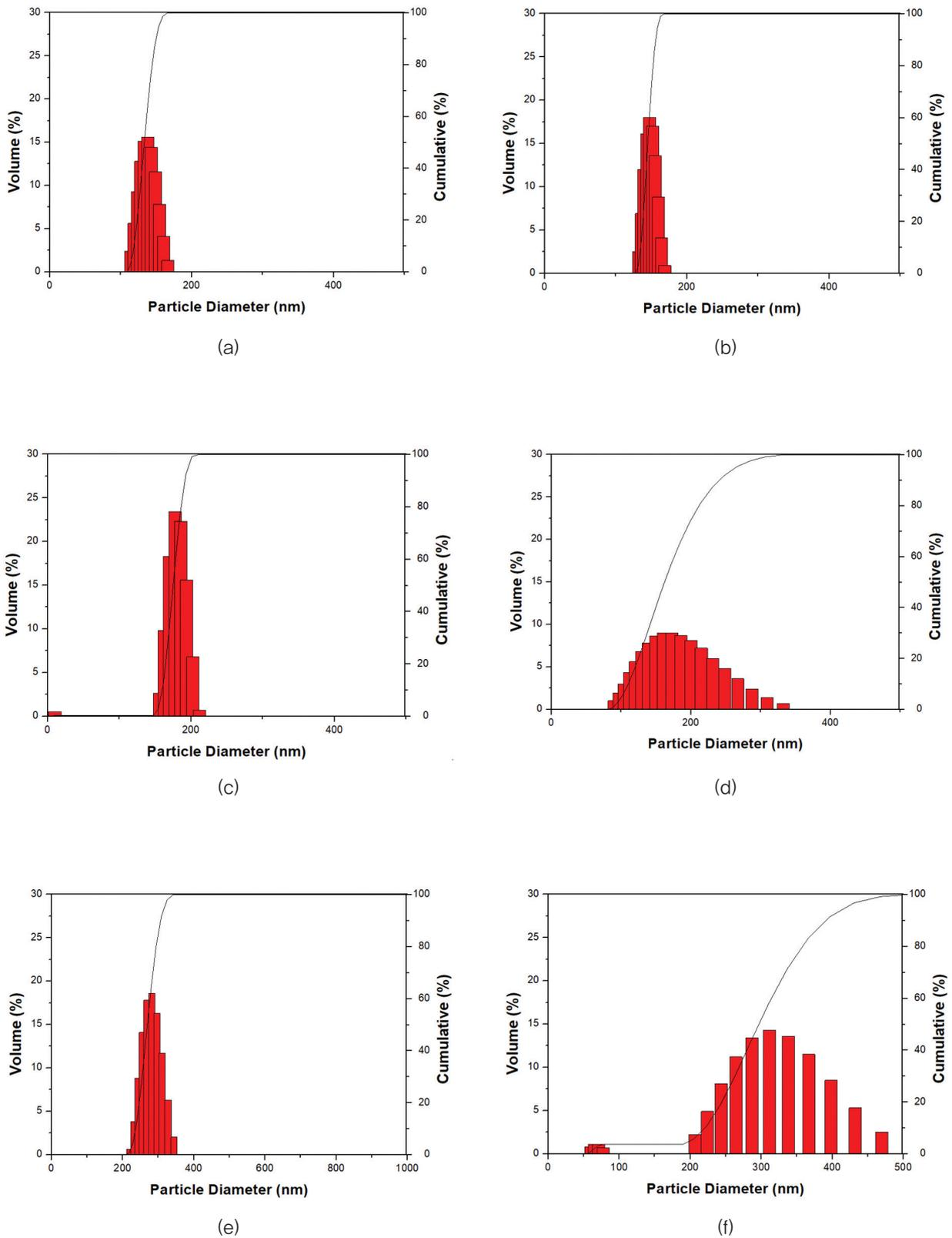
**Figure 1.** Effect of the monomer compositions on the particle size distribution of the miniemulsion polymerized binders: (a) MMA:BA=4:16, (b) MMA:BA=8:12, (c) MMA:BA=12:8, (d) MMA:BA=16:4, (e) MMA:BA:NMA:MAA=2.5:17:0.25:0.25, (f) MMA:BA:NEA:MAA=2.5:17:0.25:0.25.
