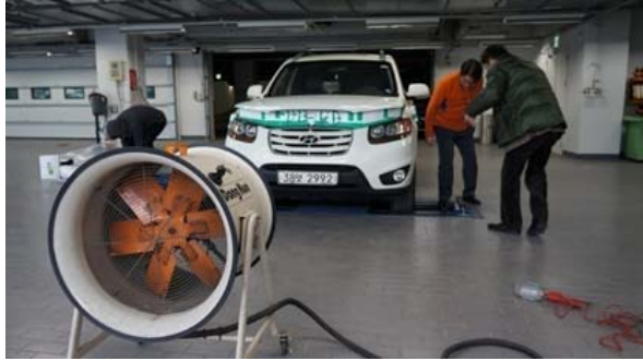
Fig. 4. Air supply device and chassis dynamo system
