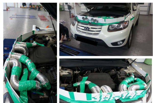
Fig. 3. Duct for cooling the components in engine room
