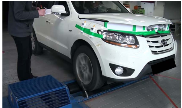
Fig. 6. Experiment through driving using chassis dynamo system
