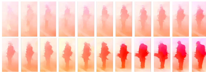
Fig. 14. Static pedestrian candidates in a dynamic environment. The effectiveness shows to be proportional to the distance to the vehicle.
