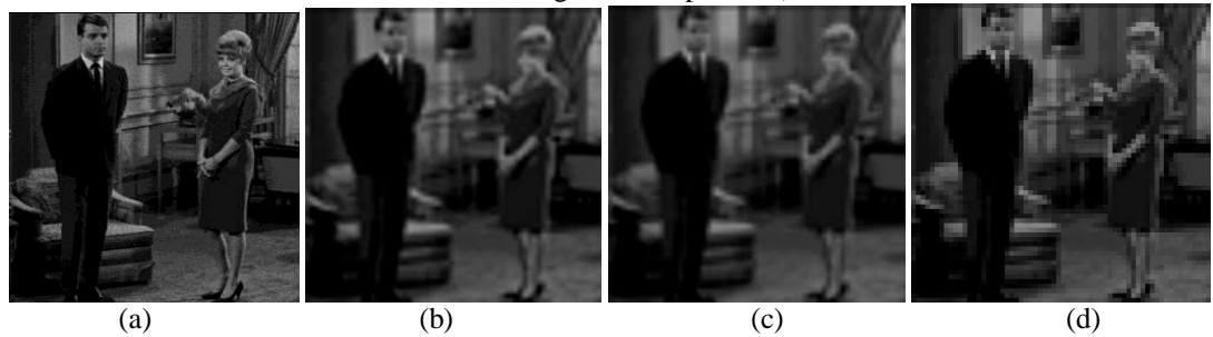
Fig. 13. Couple image reduced by the 4 times different algorithm interpolation zoom to the original sized renderings((a) Fractal interpolation (b) Bicubic interpolation (c) Double nonlinear interpolation (d) Nearestneighbor interpolation)
