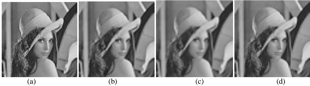
Fig. 9. Lena image reduced by the 4 times different algorithm interpolation zoom to the original sized renderings((a) Fractal interpolation, (b) Bicubic interpolation, (c) Double nonlinear interpolation, and (d) Nearestneighbor interpolation)
