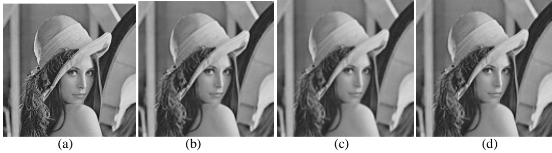
Fig. 8. Lena image reduced by the 2 times different algorithm interpolation zoom to the original sized renderings((a) Fractal interpolation, (b) Bicubic interpolation, (c) Double nonlinear interpolation, and (d) Nearestneighbor interpolation)
