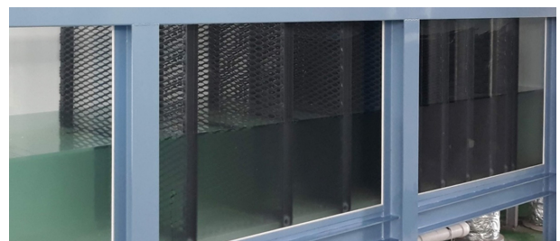
Fig. 5. A photograph of the passive absorbers at the end of the wave flume.
