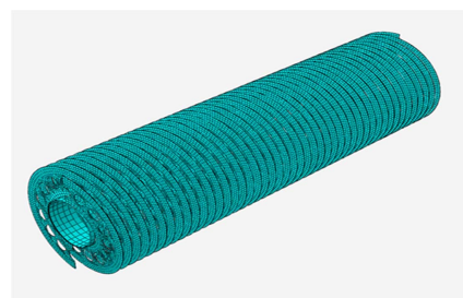
Fig. 7. Mesh of drum assembly
