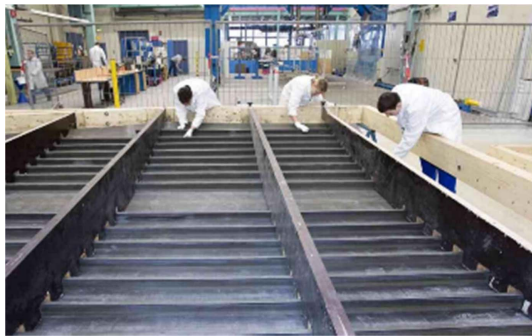
Fig. 1. A400M Cargo Door Fabrication using VAP Process [8]
