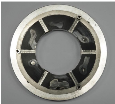
Fig. 8. Bearing specimen after load capacity test.
