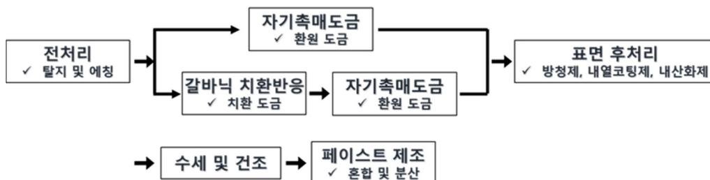
Fig. 1 Ag-coated Cu dendritic powder synthesis and paste manufacturing process
