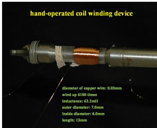
Fig. 2. Hand-operated coil, 0.03mm copper 6100 times.
