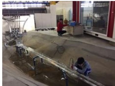
(f) Installation of an irrigation channel
