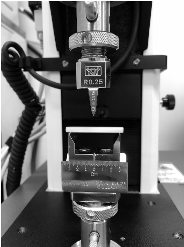
Figure 3. Specimens placed on the support span for three-point bending strength measurements
