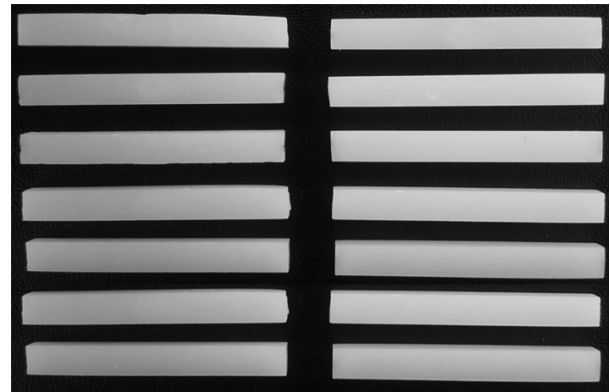
Figure 1. Low polishing group (Left): 7 specimens polished with abrasive paper of 300~1000grit. High polishing group (Right): 7 specimens polished abrasive paper of 300~2000grit.
