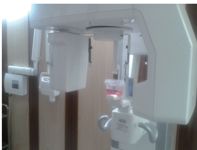
Fig. 4. Cranex 3D CBCT system. The imaging procedure using the Cranex 3D is similar to that of the NewTom 3G. However, since imaging has to be done in the standing position, the mandible was positioned similarly to how the chin is placed in a chin rest in an area compatible with scanning.
