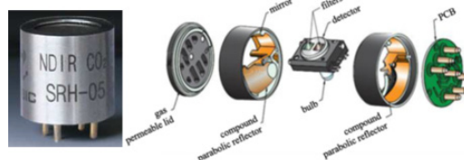
Fig. 5. Exploded View of Gas Cell
