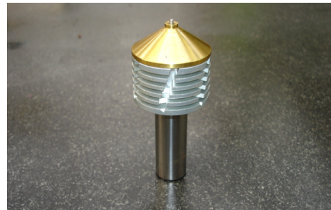
Fig. 1. Tool shape of FSW
