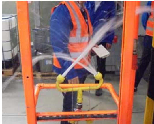
Fig. 4. Inappropriate water height by high pressure
