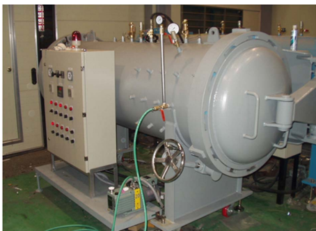
Fig. 5. High pressure heating chamber (Autoclave: 200°C, 10 atm)
