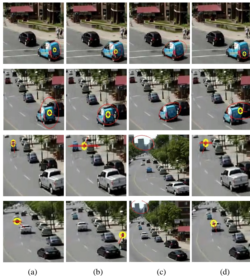
Fig. 4. Tracking captures of (a) proposed particle filter, (b) condensation particle filter, (c) camshift and (d) direction-based particle filter with T= \pi/8 in Video_2
