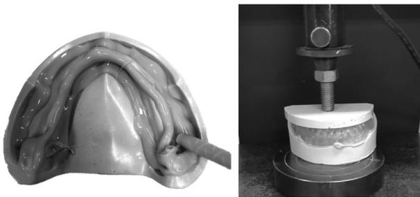
Figure 5. Pressing machine of 3.5 kgf press for silicone replica technique
