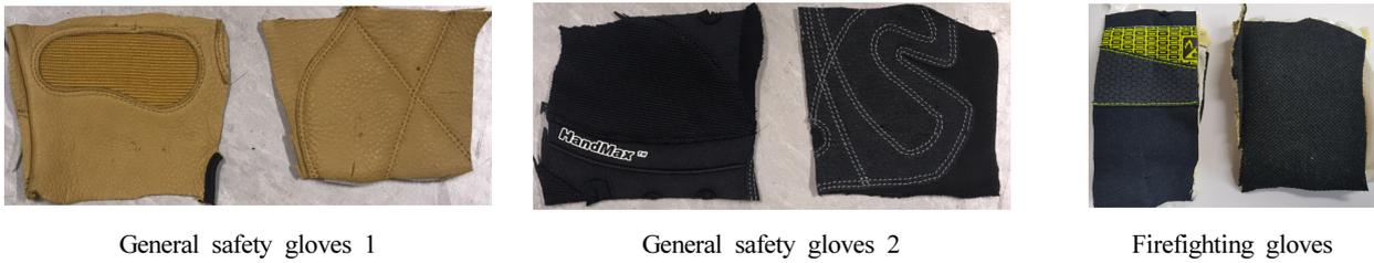
Figure 6. Conditions of safety gloves after cut and puncture resistance test.
