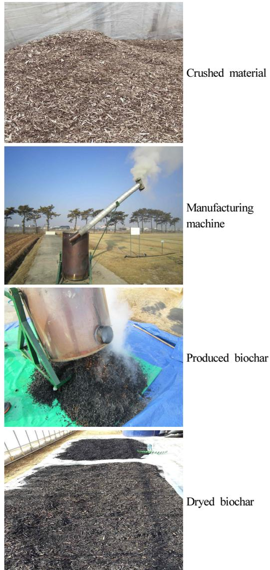
Fig. 1. The procedure of biochar using drum biochar manufacturing machine.
