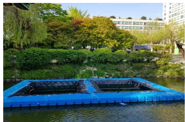
Figure 3. Selectively permeable mesh photobioreactors (SPM-PBRs) installed in Inkyung lake.
