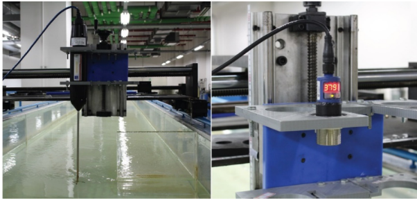
Fig. 3. ADV (left) and ultrasonic distance sensor (right)
