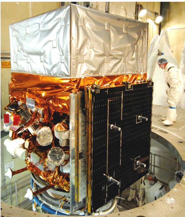
Figure 2. Fermi on the ground just before its launch. LAT is the box-shape detector on the top. The GBM detectors and the telemetry antennas can be seen on the left side. On the right side, there is the folded solar panel. (Photo courtesy: NASA FSSC)
