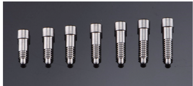
Fig. 1. A photograph of the abutment screws used in the current study. From left to right, the screws are 1.4 - 3.8 mm in length (in 0.4 mm increments) with 3.5 - 9.5 threads (in one thread increments).
