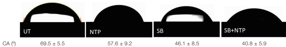
Fig. 4. Images of the contact angle (CA) after different surface treatments. UT: Untreated, NTP: Non-thermal plasma, SB: Sandblasting.
