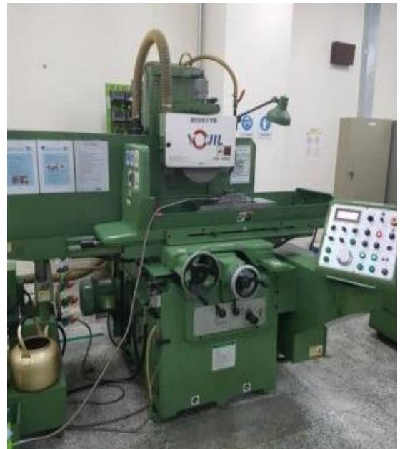
Fig. 2 Surface grinding machine
