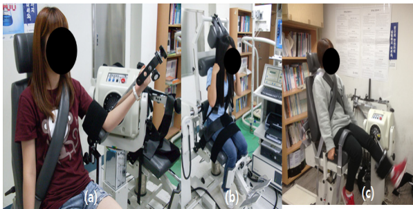
그림 6. 등속성 근 기능 평가((a)팔꿈치관절, (b)요추관절, (c)무릎관절) Fig. 6. The joint torque test for estimating muscle strength improvement((a) elbow joint, (b) lumbar exercise, (c) knee joint)
