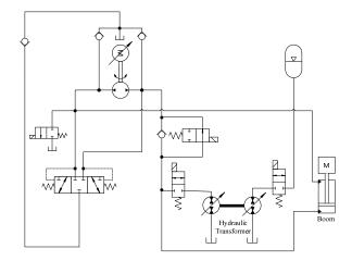
Fig. 10 The hydraulic hybrid system of using hydraulic transformer
