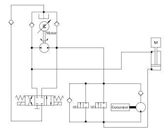
Fig. 6 One example of a hybrid hydraulic excavator
