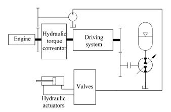
Fig. 8 Hydraulic hybrid system research by Sun Hui.
