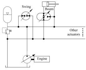
Fig. 7 Configuration of CPR system
