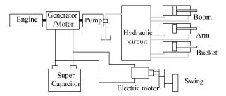
Fig. 11 The hybrid hydraulic excavator of Komatsu
