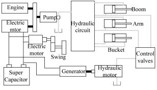
Fig. 13 ZX200 hybrid excavator of Hitachi
