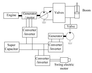
Fig. 5 The hydraulic excavator with potential energy regeneration system
