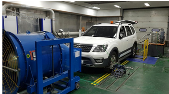
Fig. 2 Photograph of Diesel vehicles installed on chassis dynamometer
