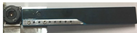
[Fig. 1] RGB-Depth-Thermal camera. The black circular (Left) and deep blue rectangular (Right) camera are the FLIR Boson Thermal and Intel R200 RGB-Depth camera, respectively [5]
