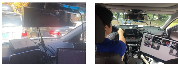
[Fig. 9] RGB-Depth-Thermal camera mounted on rearview mirror (Left) and collecting RGB-Depth-Thermal image database in vehicle (Right)
