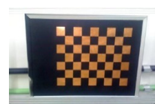
(b) Copper and high-emissive ink-based board [7]
