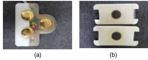
1. (a) Implemented Dry (b) AgCl electrode Fig. 1. (a) Implemented Dry (b) AgCl electrode
