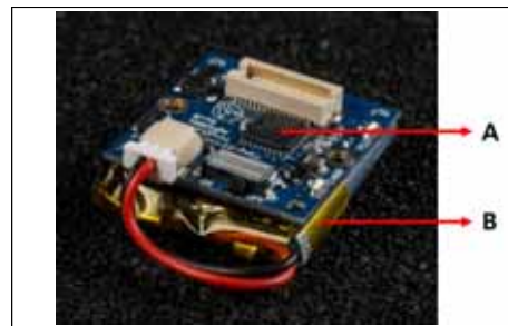
1. (A : ATMEGA 328, B: ) Fig. 1. Tinyduino Process Board (A : Microprocess ATMEGA 328, B: Battery)
