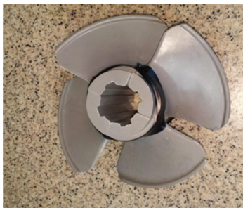
Fig. 5. Propeller using SMC method.
