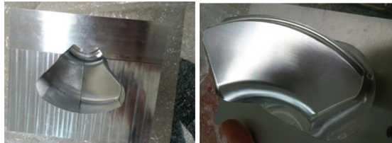
Fig. 4. Split mold production.
