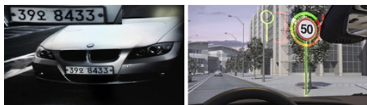
Fig. 1. Example of text detection: License plate recognition and speed limit road sign recognition
