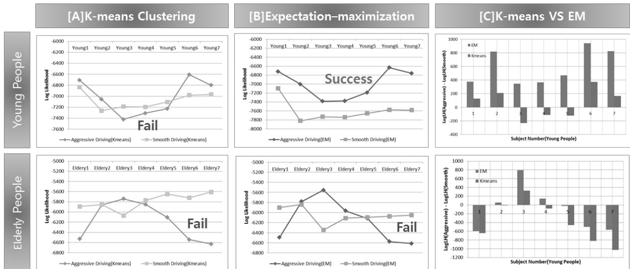
Fig. 3. The Failed Results of Aggressive Driving Data Detection with Common Clustering Method - [A] GMM Clustering with ECA [B] Expectation -Maximization with ECA [C] The Gap of Log LH(Likelihood) between Aggressive and Smooth Driving for Young/Elderly People
