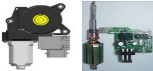
(b) Lifting motor and rpm detecting system
