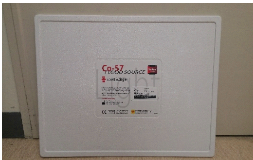
Fig. 2. 57 Co sealed source
