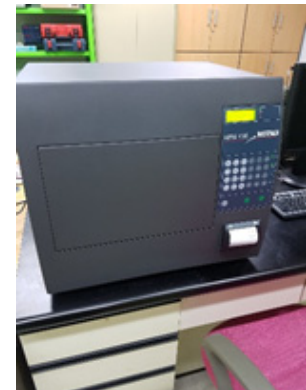
Fig. 4 Thermal conductivity measuring equipment
