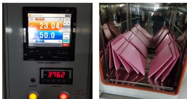
Fig. 5 Storage of thermo-hygroscopic state of insulation specimen
