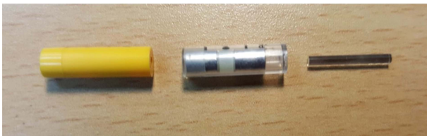
그림 3. GD-352M의 14.5 mm 길이와 보상필터와 유리소자. Fig. 3. Image of GD-352M which had low energy compensation filter was 14.5 mm in length and 4.3 mm in diameter. Tin was used as a filter material and a gap (1.5 mm in length) was made at the reading position.
