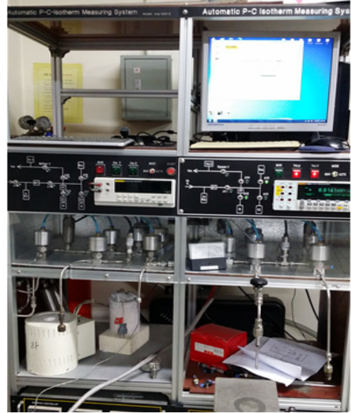
Fig. 1. Equipment for a hydrogenation of alloy
