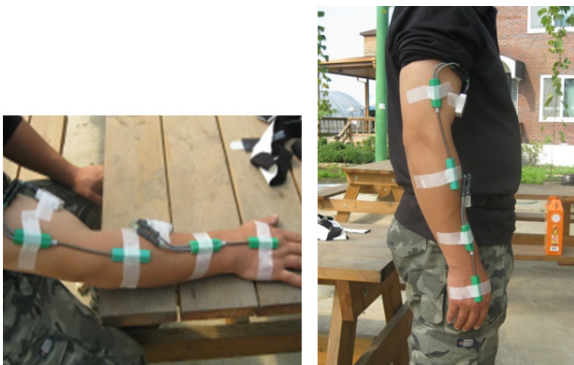
Figure 1. Attachment of goniometers on the arm and wrist
