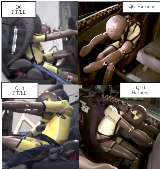
Fig. 10 Behaviors of Q6 and Q10 with pre-tensioner/load limiter and harness belt (stills from videos at the time of maximum excursion of dummy)
