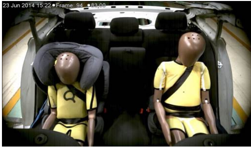
Fig. 2 Belt slippage into the neck, load limiter (stills from videos at 83ms)
