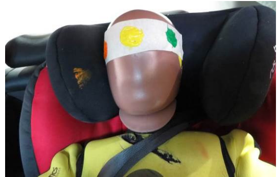
Fig. 13 Neck penetration of Q6 (after test)
