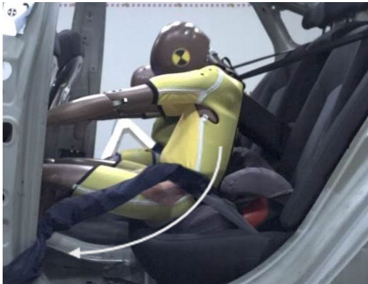
Fig. 6 Dummy sliding motion of Q10, emergency locking retractor (stills from videos at 120ms)
