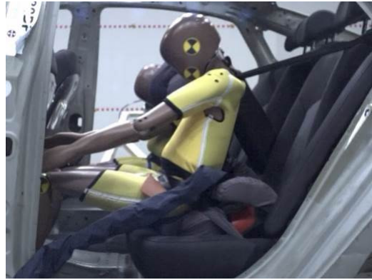
Fig. 4 Submerging of Q10, load limiter (stills from videos at 110ms)
