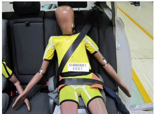
Fig. 5 Submerging of Q10, load limiter (post test)
