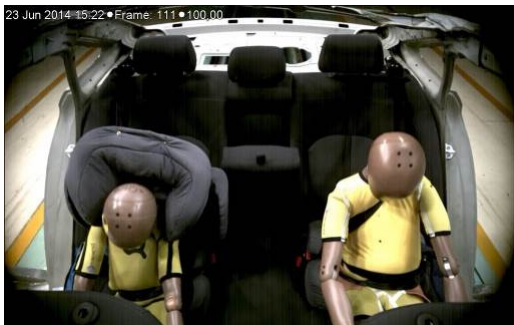
Fig. 3 Belt slippage into the neck and submerging, load limiter (stills from Videos at 110ms)
