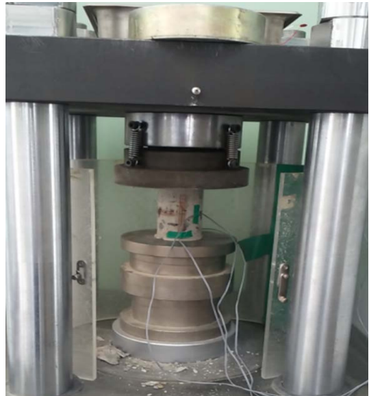
Fig. 4. The view for compressive strength test of concrete cores
