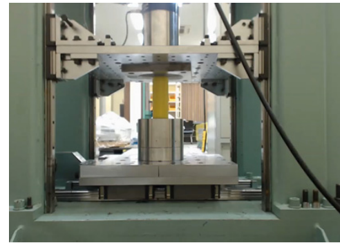
Fig. 5 MER-Spring load testing set-up
